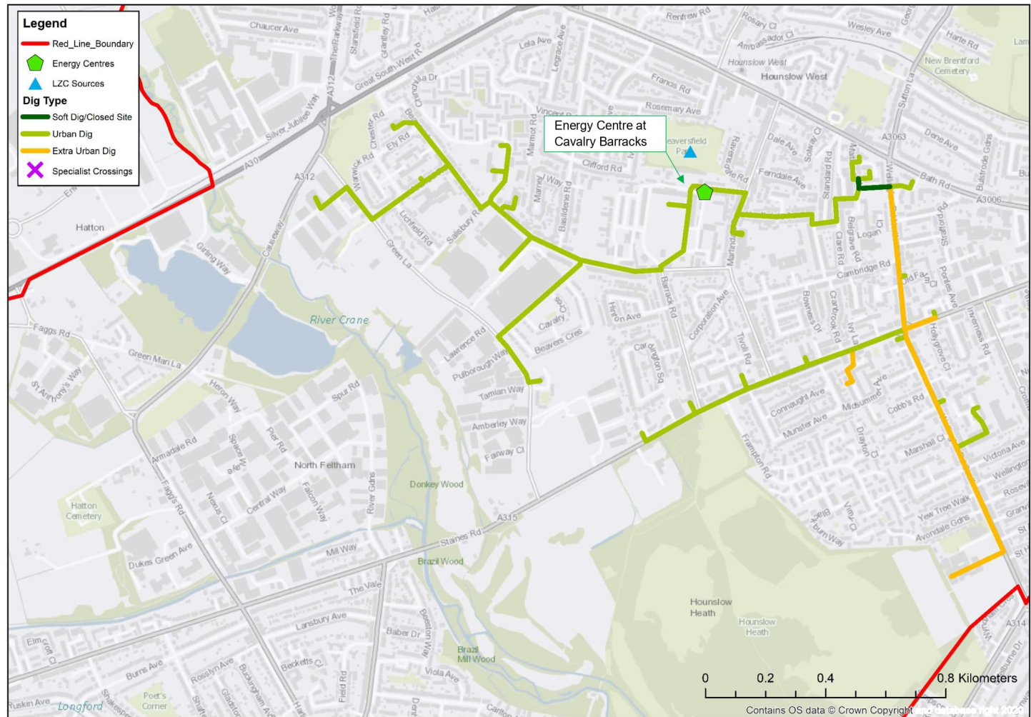
Figure 6-6: Central & Hounslow West map of distribution system, dig types and constraints
